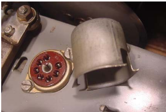
Above: The VHF RF amplifier valve base (V1) before and after 'JB Welding'
