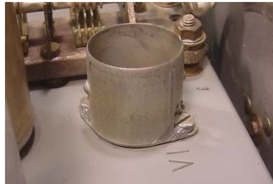
Above: The VHF RF amplifier valve base (V1) before and after 'JB Welding'
