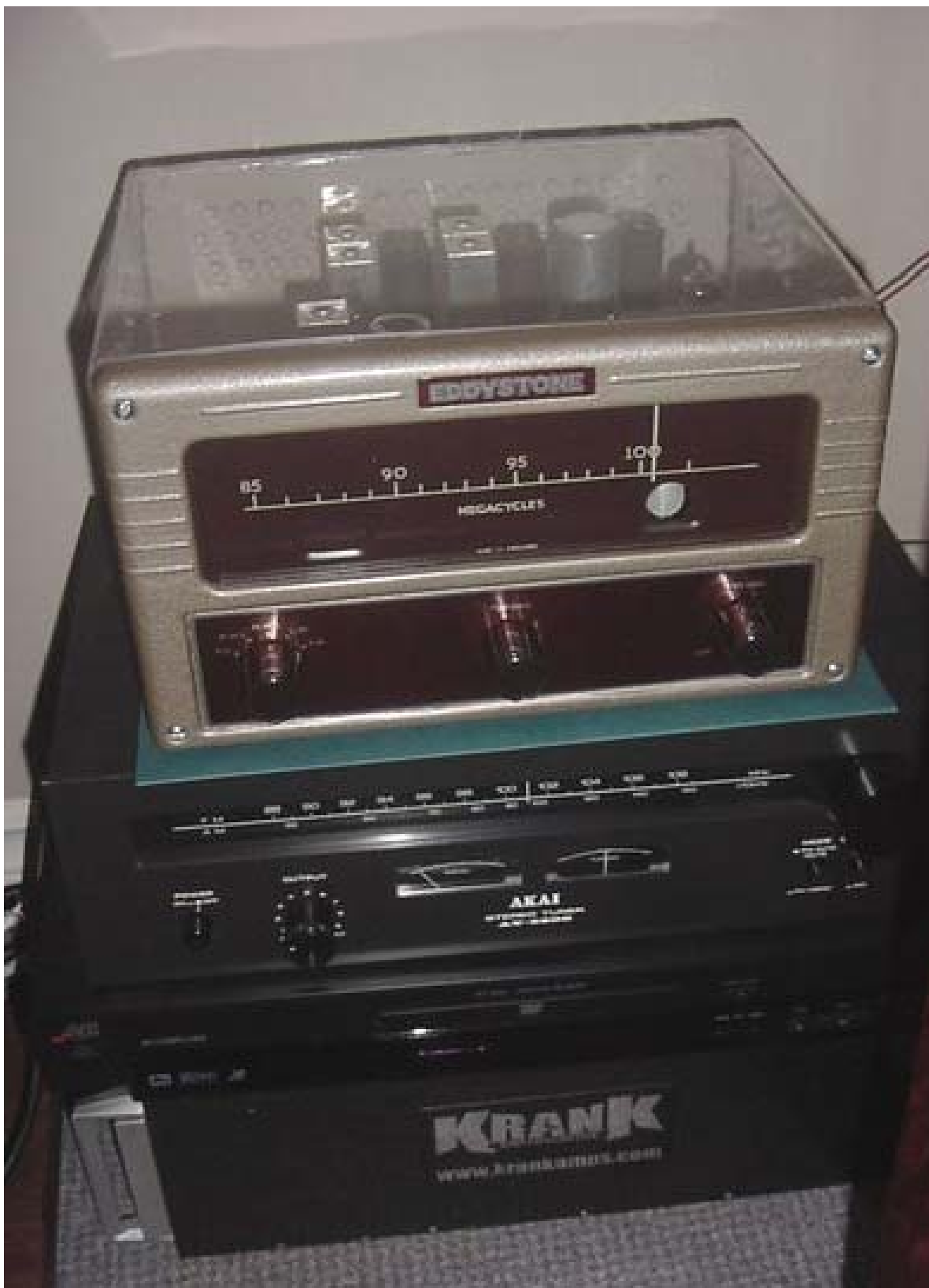
Above: Playing away quite merrily and running nice and cool too (the tuner only takes 40mA HT current, so the EZ41 runs cool, as does the power transformer)
