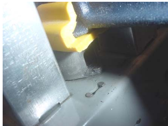
Above: The limiter stage valve base (V5) before and during 'JB Welding' (clamped)
