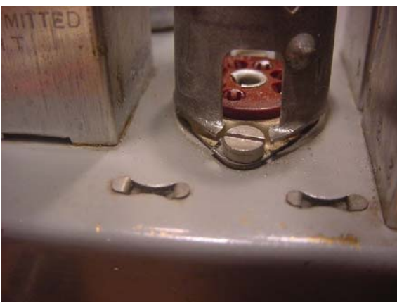
Above: The limiter stage valve base (V5) before and during 'JB Welding' (clamped)
